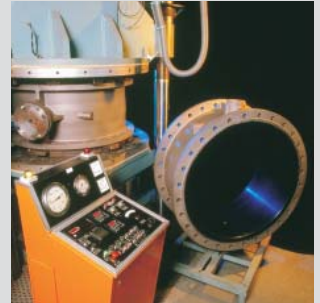
Wouter Witzel Eurovalve / AVK butterfly valves are vulcanized using the "transfer injection moulding method".
