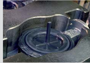
Wouter Witzel Eurovalve / AVK butterfly valves are vulcanized using the "transfer injection moulding method".
